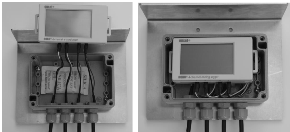
Fig. 3 Connecting dendrometers to the logger
